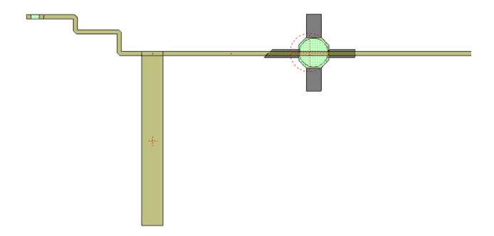
As shown above, the size of the elements that use variable "L" changes when length units change. Convert your equations' numeric values to counter the unit change.
