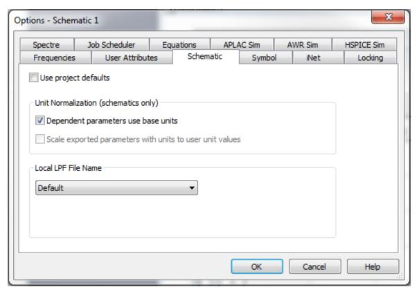
With the Dependent parameters use base units selected, length units for parameters defined by variables or equations will be in meters. Make sure you calculate your equations accordingly.
