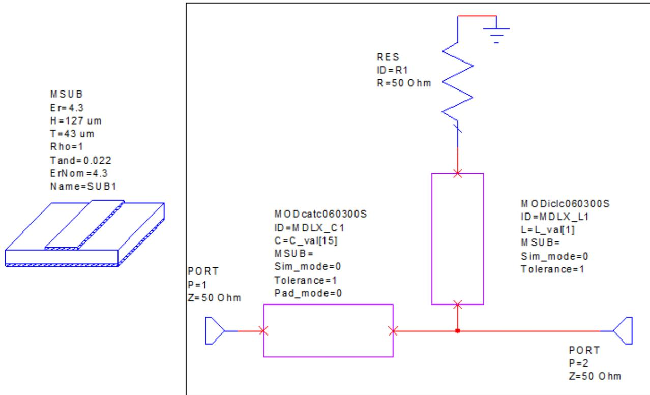
Circuit after discrete part value optimization using parasitic models.
