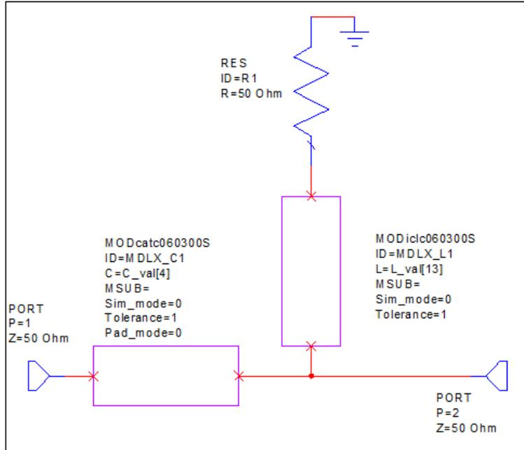
Circuit using parasitic models with values from optimized ideal model circuit.
