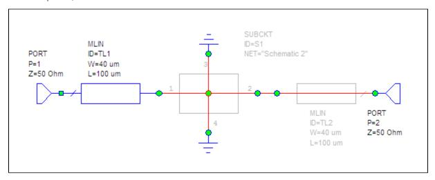
The utility can also tell the proper connectivity for coupled lines to short across the lines, not all the ports. For example, see the schematic with a selected coupled line below.
