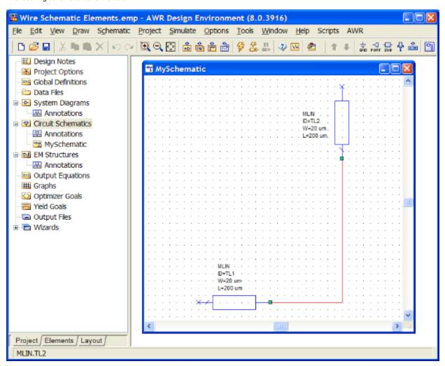
Here we've used the node objects associated with the schematic to ensure the wires connect correctly and we've added two orthogonal segments to ensure that the wires will be accepted by the schematic object.
