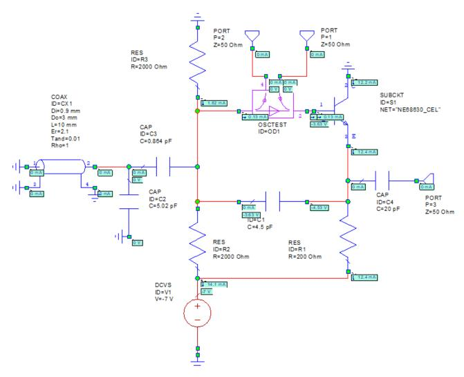
This schematic has the full design with the OSCTEST element in the feedback loop to look at the loop characteristics of this circuit. Notice that the direction of the OSCTEST element is into the transistor, which is the forward gain direction. For approximate oscillation conditions to be achieved, the angle of S21 using the OSCTEST will cross the zero angle point when the magnitude of S21 is at a maximum. The phase and magnitude of S21 are shown in the graph "Linear Oscillation Analysis".
