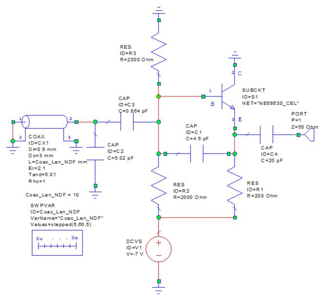
In this schematic, the oscillator circuit is drawn without additional measurement or simulation control elements, except for a SWPVAR block that varies the coax line length over a range so wide that the oscillator will not work at the extremes.
