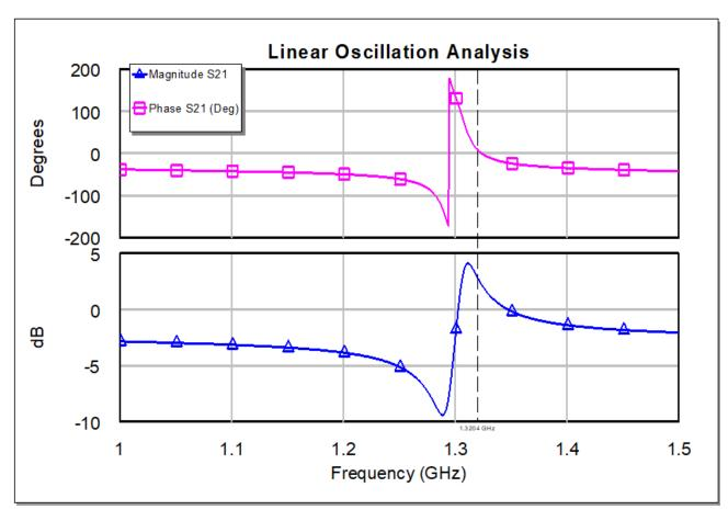
This design is very sensitive to the capacitor C1. Try tuning on its value and watch the linear results change and see how it is possible to get away from the linear oscillation approximation. The original design value is 4.5 pF. Notice with the marker that the approximate oscillation frequency with this circuit is 1.32 GHz.
