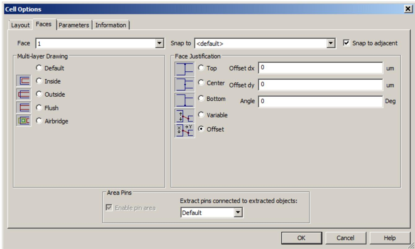
The default setting for the Face Justification setting is Center. By changing this setting to Offset you can now enter offset values for x, y and an angle. After any changes, rat lines will draw to this new location and snapping will also use this new location.
